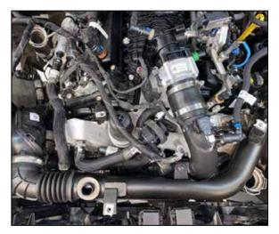
5. Loosen the hose clamps that secure the driver's side intake tube.
