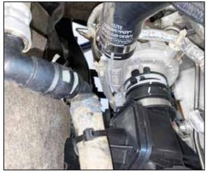
10. Remove the bolt on the bottom side of the passenger side intake tube that secures the tube to the engine. Then release the spring clamp that secures the intake tube to the turbo and remove the passenger side intake tube.
