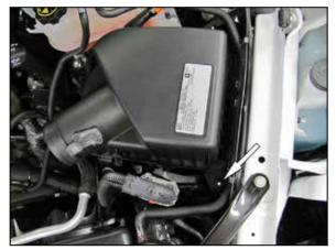
9. Remove the nut that secures the air filter housing assembly to the vehicle. Remove the air filter housing assembly from the vehicle. **NOTE:** Go slow and use caution to remove the housing. It is indexed into two holes in the rear with rubber grommets that can fall off easily and be lost. It is a tight fit but will come out without being forced.
