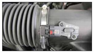
2. Disconnect the mass air sensor electrical connection.
