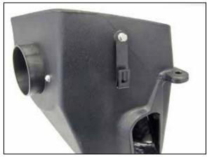
12. Install the provided wiring harness bracket onto the  $K\&N^{\circ}$  air filter housing and secure with the provided hardware.
