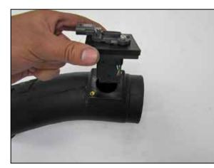
20. Install the mass air sensor assembly into the K&N<sup>®</sup> intake tube in the direction shown and secure with the provided hardware.
