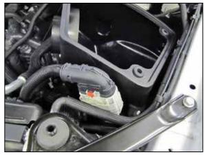
16. Clip the wiring harness onto the bracket installed onto the  $K\&N^{\mbox{\tiny (B)}}$  air filter housing.
