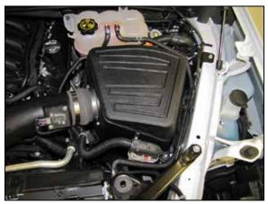
27. Install the K&N<sup>®</sup> air filter housing lid onto the air filter housing so the posts engage with the mounting grommets.
