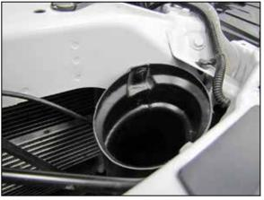
15. Push the factory fresh air intake duct into the  $K\&N^{\circ}$  air filter housing and then reinstall the plastic clip to secure it into position.
