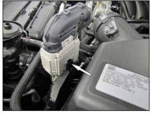
8. Using a small 90° pick or similar tool, release the locking tap that secures the wiring harness bulk connector to the air filter housing and then unhook the connector from the bouving
