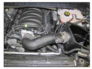
22. Install the K&N<sup>®</sup> intake tube into the coupler at the air filter housing and then into the coupler on the throttle body, adjust the tube for best fit and then secure with the provided hose clamps.
