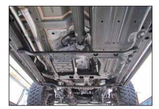
10. Reinstall the transfer case skid plate and secure with the factory bolts.
