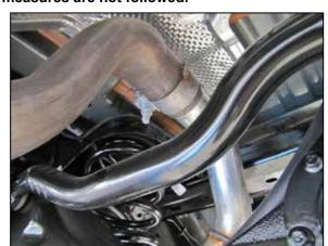
2. Loosen the clamp that secures the muffler pipe to the exhaust pipe.
