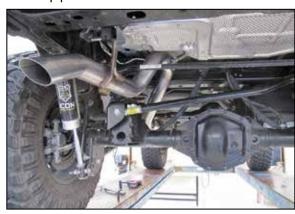
16. Check alignment and reposition as necessary. Once final position is satisfactory, tighten all band clamps from front to rear of vehicle.
