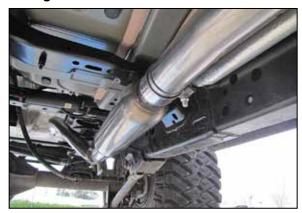
12. Install the K&N® muffler onto the K&N® mid pipe and into the factory hanger.
