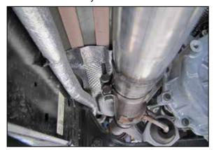
11. Install the K&N® mid pipe to the factory catalyst pipe and secure with the factory clamp.
