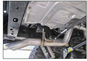
15. Install the K&N® tail pipe onto the K&N® exhaust pipe.
