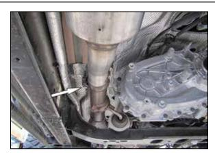
7. Loosen the clamp the secures the exhaust mid pipe to the exhaust catalyst pipe.
