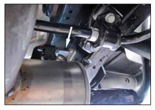
4. Loosen and remove the two bolts that secure the passenger side muffler hanger to the chassis.
