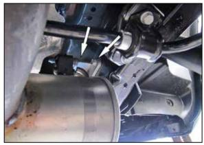
3. Loosen and remove the two bolts that secure the driver side muffler hanger to the chassis.
