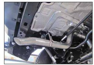
8. Install the K&N® tail pipe onto the factory exhaust pipe.
