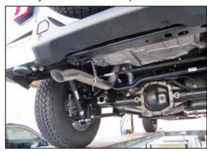
11. Check alignment and reposition as necessary. Once final position is satisfactory, tighten all band clamps from front to rear of vehicle.
