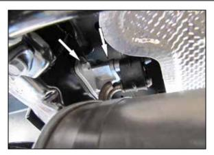
4. Loosen and remove the two bolts that secure the passenger side muffler hanger to the chassis. NOTE: one bolt is not in view in this picture. Support the muffler assembly while removing the bolts as it may now swing and fall.
