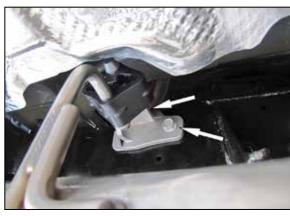
10. Secure the hanger to the factory location using the factory bolts removed in step #3.
