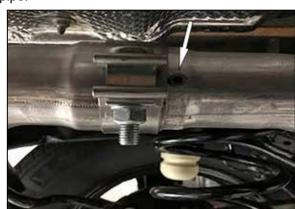
9. Make sure the K&N® tailpipe rests up against the clocking feature on the factory mid-pipe.
