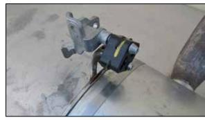
6. Remove the driver side muffler hanger from the stock muffler.
