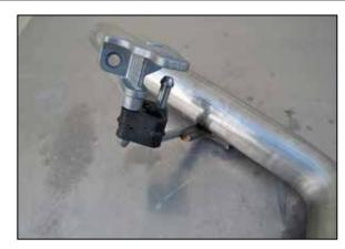
7. Install the driver side muffler hanger onto the K&N® tail pipe hanger.
