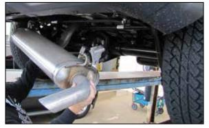
5. Using a twisting motion so the muffler pipe slides off the exhaust pipe, remove the muffler assembly from the vehicle.
