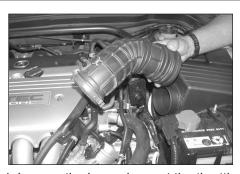
4. Loosen the hose clamp at the throttle body and remove the stock intake tube as shown.
