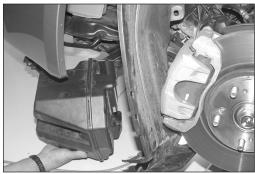
14. Remove the resonator as shown.
