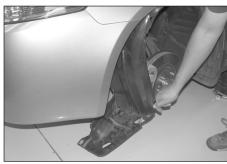
9. Remove the two bolts and three plastic rivets, then, lower the inner fender valance as shown.
