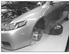
7. Lift the vehicle up and support it with jack stands and remove the front side drivers tire as shown.
