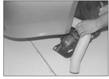
25. Install the cold air tube from underneath the vehicle as shown.
