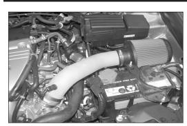
33. This K&N® high flow intake system has been designed to be used in two different configurations. In the case of inclement weather, the cold air tube can be removed and the air filter can be clamped onto the intake tube located in the engine compartment to avoid the possibility of ingesting water into the engine.
