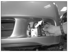
12. Loosen and remove the bolt secures the resonator to the inner fender as shown.
