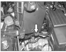
6. Lift the air cleaner assembly upwards, then, unclip the wire harness from the tab on the air cleaner assembly as shown.
