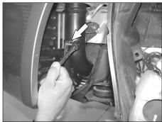
10. Loosen and remove the bolt that secures the air inlet tube to the resonator as shown.
