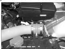
24. Install the silicone hump hose and hose clamps onto the K&N® short ram tube as shown.
