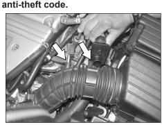
2. Disconnect the crankcase vent hose and the EVAP vent hose from the stock intake tube as shown.
