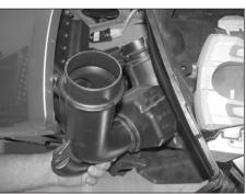
13. Remove the air inlet duct as shown.
