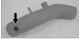
17. Install the provided grommet into the  $K\&N^{\otimes}$  short ram tube as shown.
