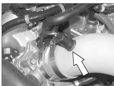
23. Insert the air temperature sensor into the grommet on the K&N® short ram tube as shown.
