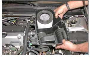
11. Pull upwards to remove the lower air cleaner assembly as shown.
