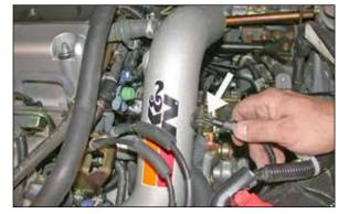
23. Push the air temperature sensor into the grommet on the K&N<sup>®</sup> intake tube as shown.
