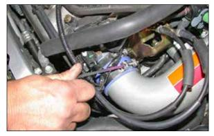
21. Using a flat blade screwdriver, tighten the hose clamp on the silicone hose as shown.
