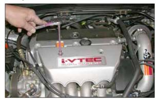
26. Reinstall the engine cover as shown.
