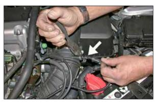
4. Using a pair of pliers, depress the hose clamp and remove the air temperature sensor from the stock intake tube as shown.
