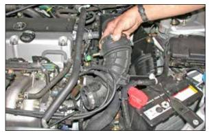
9. Pull the stock intake tube off of the throttle body, then remove the stock intake tube as shown.
