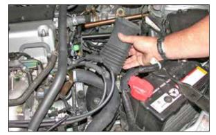
13. Remove the air inlet duct as shown. NOTE: K&N Engineering, Inc., recommends that customers do not discard factory air intake.
