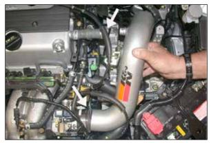
18. Install the second hose clamp onto the silicone hose, then, slide the K&N<sup>®</sup> intake tube into the silicone hose as shown. Line up the intake tube bracket with the original air cleaner mounting point.
