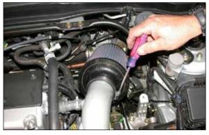
24. Install the K&N<sup>®</sup> air filter onto the K&N<sup>®</sup> intake tube and secure with the provided hose clamp as shown.
