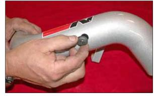
17. Install the provided grommet into the hole on the K&N $^{\mbox{\tiny 0}}$  intake tube as shown.
