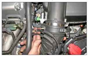
6. Remove the Idle air bypass control thermal valve vent hose from the vent on the stock intake tube as shown.
