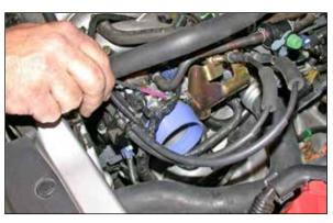
16. Install the silicone hose and hose clamp onto the throttle body as shown.
