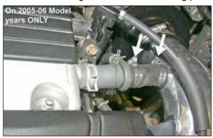
19. **2005-06 Model Year Vehicles ONLY:** Using the supplied silicone hose and hose clamps, secure the silicone hose to the stock crank case vent line and to the vent tube on the intake tube as shown.
