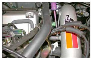
22. Reconnect the idle air bypass control thermal valve vent hose to the vent on the K&N<sup>®</sup> intake tube and secure with the provided hose clamp as shown.
