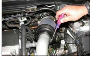
24. Install the K&N® air filter onto the K&N® intake tube and secure with the provided hose clamp as
