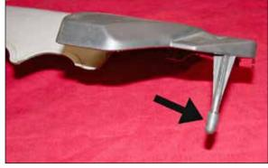
25. Install the rubber cap plug onto the stand off on the engine cover as shown.
