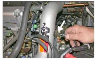
23. Push the air temperature sensor into the grommet on the K&N® intake tube as shown.
