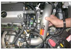
18. Install the second hose clamp onto the silicone hose, then, slide the K&N® intake tube into the silicone hose as shown. Line up the intake tube bracket with the original air cleaner mounting point.
