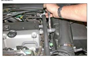
3. Using a pair of pliers, depress the hose clamp and slide it back off of the crank case vent on the air cleaner assembly as shown.
