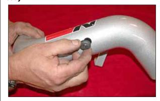
17. Install the provided grommet into the hole on the K&N® intake tube as shown.
