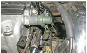
14. **2005-06 Model Year Vehicles ONLY:** On '05-'06 models, remove the stock crank case vent hose as shown.
