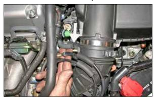
6. Remove the Idle air bypass control thermal valve vent hose from the vent on the stock intake tube as shown.
