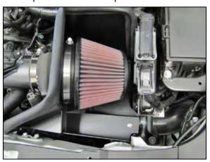
Install the K&N® air filter onto the filter adapter and secure with the provided hose clamp.
