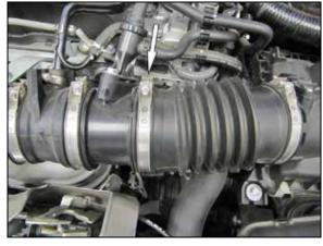
3. Loosen the hose clamp that secures the intake hose to the turbo inlet tube.
