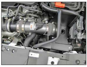
14. Install the K&N® intake tube into the coupler at the filter adapter and align with the turbo inlet pipe, slide the coupler back onto the turbo inlet pipe and adjust the tube for best fit. Secure the intake tube with the provided hose clamps.
