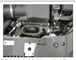
5. Remove the two bolts that secure the air filter housing to the inner fender and then remove the bolts from the vehicle.
