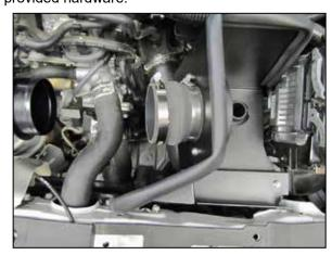
11. Install the provided coupling hose (087121) onto the filter adapter and secure with the provided hose clamp.
