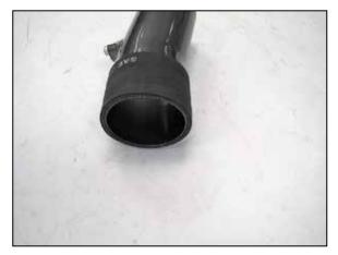
12. Install the provided coupling hose (08711) onto the intake tube so that id slides all the way on. Do not secure the hose now.
