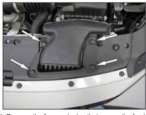
4. Remove the four push pins that secure the fresh air intake duct and then lift the fresh air intake duct out to remove it from the vehicle.
