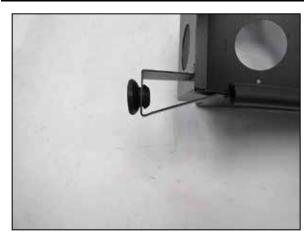
7. Remove the mounting grommet from the factory air filter housing and install it into the K&N® heat shield as shown.
