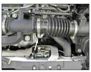
3. Loosen the hose clamp that secures the intake tube to the turbo inlet pipe.
