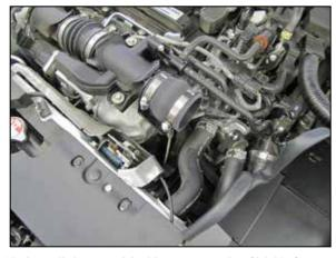
12. Install the provided hump coupler (08487) onto the turbo inlet and secure with the provided hose
