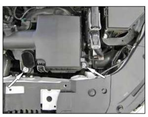
5. Remove the two bolts that secure the air filter housing and then lift up the intake assembly to remove it from the vehicle.
