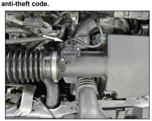
2. Disconnect the mass air sensor electrical connection.
