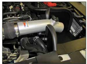
13. Install the K&N® intake tube into the coupler at the turbo inlet and then align the mounting stud with the hole in heat shield. Adjust the intake tube for best fit and then secure with the provided hardware and hose clamp.
