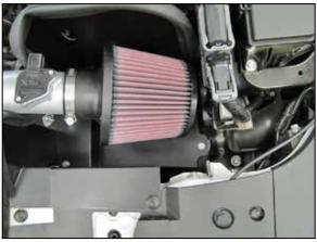
14. Install the K&N® air filter and secure with the provided hose clamp.
