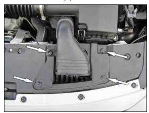
4. Remove the four pins that secure the fresh air intake to the core support. Remove the fresh air duct from the vehicle.
