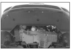
13c. On vehicle's that were equipped with the splash shield, reinstall with the bolts removed in step #8b.
