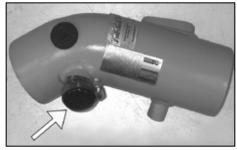
19c. On vehicles not equipped with an air injection pump, install the provided caplug onto the air injection fitting and secure with the provided hose clamp as shown.
