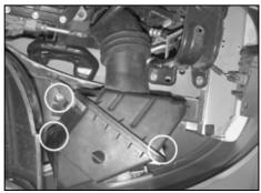
9. Remove the three bolts that fasten the lower airbox to the inner fender well.
