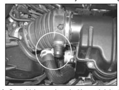
3. On vehicles equipped with an air injection pump; using pliers, release the spring clamp that fastens the air injection hose to the stock intake tube. Disconnect the air injection hose from the stock intake tube.
