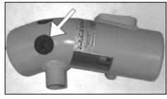
19b. On vehicles equipped with an EVAP vent line, install the provided grommet into the hole drilled in step #19a.
