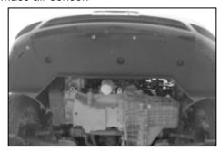
8b. On vehicles equipped with the splash shield, remove the six bolts and five black plastic screws which secure the splash shield to the bumper cover, then remove the splash shield from the vehicle.
