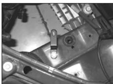
17. Install the heat shield mounting bracket (06488) onto the inner fender; fasten using the provided hardware.
