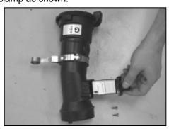
20. Remove the two screws that fasten the mass air sensor to the mass air sensor housing, then remove the mass air sensor from the housing.
