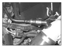
27. Connect the crankcase vent hose to the stock fitting previously installed into the K&N® intake tube.
