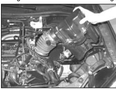
5. Loosen the hose clamp at the throttle body, then lift firmly, separating the upper intake housing from the mass air sensor housing and throttle body. Remove the upper intake housing.
