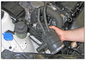
6. Loosen the hose clamp securing the intake tube to the turbo inlet, then remove the intake tube from the vehicle.
