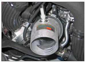
9. Install the K&N<sup>®</sup> intake tube into the silicone hose and secure with the provided hose clamp. **NOTE: Do not completely tighten the hose clamp at this time.**
