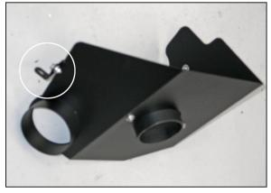
12. Install the provided "L" bracket (070066) onto the heat shield as shown using the provided hardware.
