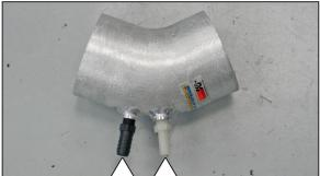
2. Loosen the hose clamp securing the intake tube to the airbox, then disconnect the tube from the airbox.
