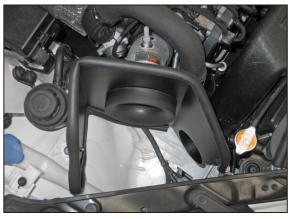
15. Set the heat shield assembly into the engine compartment so the silicone hose slips onto the intake tube and the fresh air duct slips over the tube attached to the heat shield. Align the intake tube and hoses, then tighten the hose clamps and secure the heat shield brackets to the airbox mounting locations using the provided hardware.
