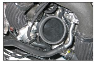
7. Install the elbow silicone hose (08504) onto the turbo inlet as shown and secure with the provided hose clamp.
