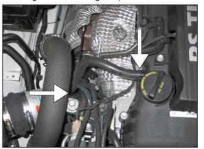
16. Install the  $\frac{1}{2}$ "ID silicone vent hose onto the valve cover port. Connect the opposite end of the vent hose to the  $\frac{1}{2}$ "OD vent fitting installed in the intake tube.
