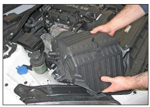
4. Remove the airbox assembly from the vehicle. NOTE: K&N Engineering, Inc., recommends that customers do not discard factory air intake.
