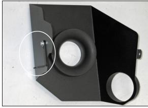
11. Install the provided "L" bracket (070742) onto the heat shield as shown using the provided hardware.
