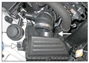
3. Remove the three bolts securing the airbox to the inner fender.
