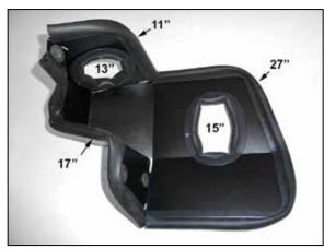
9. Install the cut edge trim onto the heat shield as shown.
