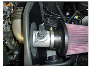
16. Reconnect the mass air sensor electrical connection.
