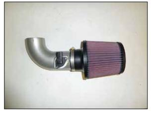
12. Install the air filter onto the K&N® intake tube and secure with the provided hose clamp. NOTE: Drycharger® air filter wrap; part # RX-4990DK is available to purchase separately. To learn more about Drycharger® filter wraps or look up color availability please visit http://www.knfilters.com®.
