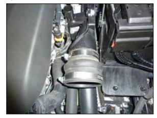
13. Install the hump coupler (5-574) onto the turbo inlet pipe and secure with the provided hose clamp.
