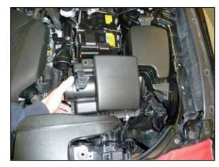
5. Pull straight up on the air filter housing assembly and remove it from the vehicle.
