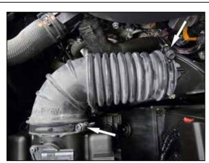
3. Loosen the clamps that secure the factory intake hose and then remove the factory hose from the vehicle.
