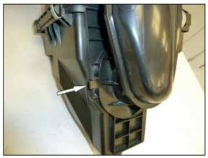
6. Lift the locking tab and then rotate the fresh air scoop counter clockwise to remove it from the air filter housing.
