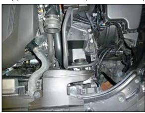
14. Install the heat shield assembly into the vehicle so the mounting grommets secure over the factory mounting studs. Secure the fresh air scoop with the factory bolts
