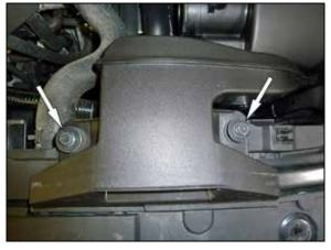
4. Remove the two bolts that secure the fresh air intake scoop to the core support.
