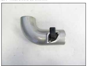
11. Remove the mass air sensor from the factory air filter housing and install it into the K&N® intake tube and secure with the provided hardware.
