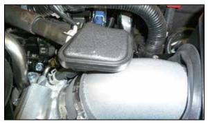
18. Install the PVC chamber into the grommet in the K&N $^{\circ}$  intake tube.
