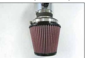
16. Install the K&N<sup>®</sup> air filter onto the filter adapter and secure with the provided hose clamp.
