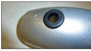
14. Install the provided grommet into the K&N<sup>®</sup> intake tube.
