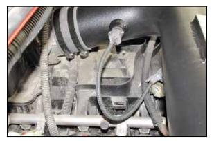
28. Connect the provided extension harness to the factory inlet air temperature sensor harness and then connect the open end to the sensor installed into the K&N<sup>®</sup> intake tube.
