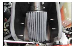
29. Install the air filter and secure with the provided hose clamp.
