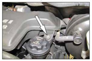
6. Loosen the remaining bolt securing the intake plenum.
