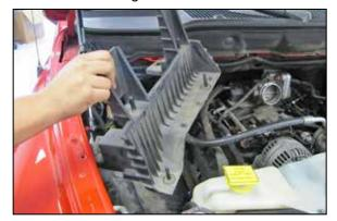
10. Remove the four bolts that secure the air filter mounting bracket and then remove the bracket from the vehicle.
