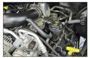
27. Install the provided crank case vent hose onto the valve cover port and then connect the open end to the intake tube.
