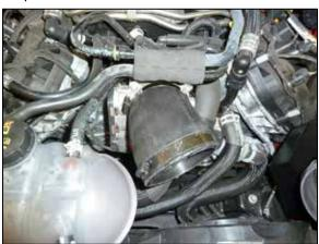
14. Install the provided angled coupler hose (5-1100) onto the throttle body and secure with the provided hose clamp
