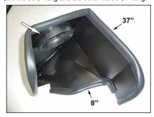
9. Install the provided edge trim onto the K&N® heat shield as shown. Install the air filter adapter into the heat shield and secure with the provided hardware.
