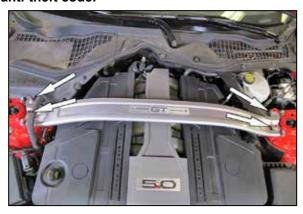
2. Remove the four nuts that secure the strut tower brace and then remove the strut tower brace from the vehicle.
