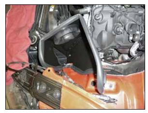
12. Install the heat shield assembly onto the inner fender and secure with the provided hardware.
