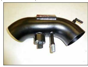
15. Install the Provided 90° fitting into the K&N® intake tube. Remove the mass air sensor from the factory housing and install it into the K&N® intake tube using the provided hardware.
