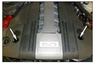
3. Remove the fastener covers on the engine cover, remove the two nuts that secure the cover and then remove the cover from the engine.
