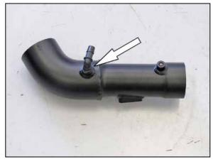
19. Install the provided  $90^{\circ}$  NPT vent fitting into the driver's side K&N<sup>®</sup> intake tube (27466) as shown. NOTE: Plastic NPT fittings are easy to cross thread. Install the vent fitting "hand" tight, then turn it two complete turns with a wrench.
