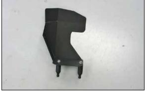
29. Install the two heat shield mounting pins onto the passenger side heat shield (074058) and secure with the provided hardware.
