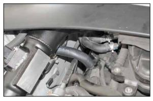
38. Install the 5" crank case vent hose onto the 90° fitting on the K&N® intake tube and then attach the open end to the vent port on the valve cover. NOTE: Choose the appropriate size hose and fitting for your application. Some models vary between 1/2" and 5/8".
