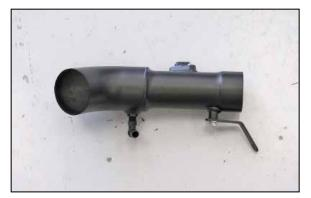
22. Install the tube mounting bracket onto the driver's side K&N<sup>®</sup> intake tube as shown and secure with the provided hardware. NOTE: The part number of the bracket will be on the leg pointing down away from the intake tube when installed properly.
