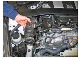
8. Remove the right side intake hose from the vehicle.
