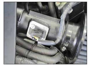
40. Reconnect the mass air sensor electrical connection.
