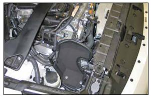
32. Install the heat shield assembly into the vehicle so that the mounting pins engage into the air box mounting grommets.
