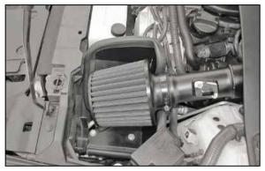
26. Install the K&N<sup> $\otimes$ </sup> air filter onto the K&N<sup> $\otimes$ </sup> intake tube and secure with the provided hose clamp.
