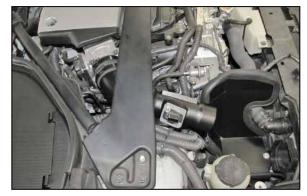
with the hose clamp to the 90° vent fitting on the driver's side  $K\&N^{\odot}$  intake tube and then connect the other end to the vent port on the valve cover. **NOTE: Some trimming of the crank case vent hose may be necessary.**
