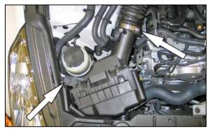
4. Loosen the hose clamp which secures the passenger side intake hose to the air box. Remove the bolt which secures the air box to the inner fender.
