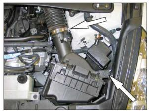
10. Loosen the hose clamp which secures the right side intake hose to the air box. Remove the bolt
