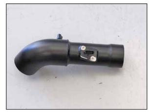
21. Install the mass air sensor into the driver's side  $K\&N^{\textcircled{o}}$  intake tube and secure with the provided hardware.
