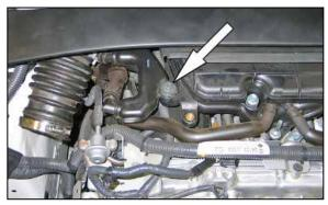
6. Remove the bolt shown which secures the crank case vent tube assembly to the intake plenum.
