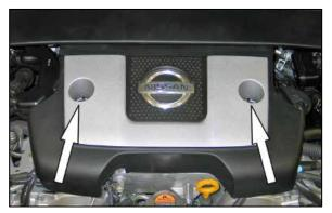
2. Remove the two bolts which secure the front engine cover and then remove the front engine cover. 3. Disconnect the passenger side mass air sensor and unhook the wiring harness from the air box.
