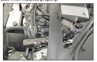
23. Install the K&N<sup>®</sup> intake tube into the silicone hose at the throttle body and align the bracket with the mounting hole in the heat shield. Adjust the tube and heat shield for proper fit and then secure with the provided hardware and hose clamp. **NOTE: The tube mounting bracket is to be attached on the back side of the heat shield.**
