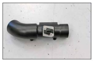
35. Install the mass air sensor into the passenger side K&N $^{\circ}$  intake tube and secure with the provided hardware.
