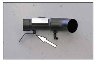
36. Install the tube mounting bracket onto the passenger side K&N<sup>®</sup> intake tube as shown and secure with the provided hardware. NOTE: The part number of the bracket will be on the leg pointing down from the intake tube when installed properly.
