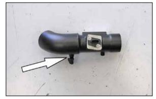
33. Install the provided 90° NPT vent fitting into the K&N^{\mbox{\tiny 6}} intake tube (27642) as shown.
