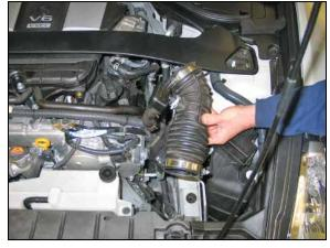
13. Remove the driver's side intake hose from the vehicle.
