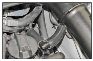
25. Connect the end of the crank case vent hose
