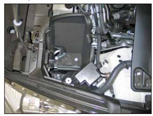
18. Install the heat shield assembly into the vehicle so that the mounting pins engage into the air box mounting grommets.
