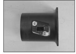
14. On 2006 models, install the mass air sensor removed in step #13 into the mass air sensor housing with the supplied hardware as shown.
