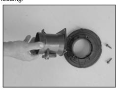
12. On 2005 and earlier vehicles, remove the two bolts that secure the mass air sensor to the mounting plate and then remove the sensor as shown.
