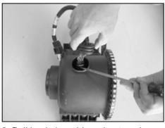
10. Pull back the rubber plug to gain access to the primary mass air sensor connection. Using a small screw driver, release the locking tab and disconnect the mass air sensor electrical connection.
