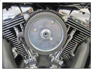
9. Install the filter onto the base plate and secure with the provided hardware.
