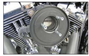
7. Install the filter spacer bolts through the filter back plate and then install the gasket onto the spacer bolts passed through the back plate. Install the filter back plate assembly onto the breather plate and secure with the filter spacer bolts.
