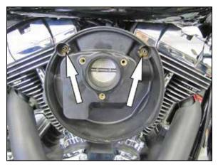
4. Remove the two crank case breather bolts shown and then remove the air filter base from the throttle body.
