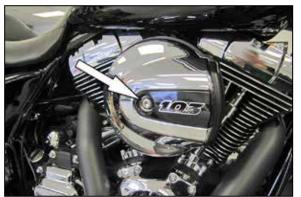
2. Remove the bolt which secures the bonnet to the filter assembly and then remove the bonnet from the vehicle.
