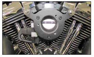
6. Install the crank case breather plate along with the two remaining O-rings, breather bolts, throttle body mounting bolts and throttle body gasket as shown.
