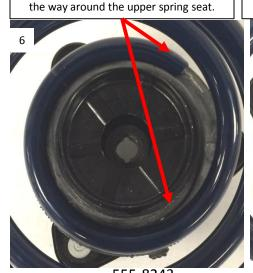
Correct, notice how the coil wraps 3/4 of
