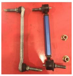
Figure 2: Factory vs Steeda front swaybar endlinks
