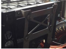
muffler and muffler bracket, you may need to loosen the head pipe bolts and swing it in the desired direction. Be sure to re-tighten the head pipe bolts before mounting the muffler\*\*\*
